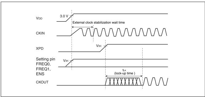
When XPD pin controls the power-down, stable clock is output from CKOUT pin after becoming XPD pin = "H" level (in the maximum after lock-Up time  $(t_{LK})$ ).
