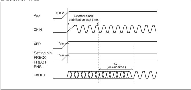
If the XPD pin is fixed at the "H" level, the maximum time after the power is turned on until the set clock signal is output from CKOUT pin is (the stabilization wait time of input clock to CKIN pin) + (the lock-up time "tlk"). For the input clock stabilization time, check the characteristics of the resonator or oscillator used.
